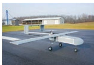
The SPAARO Unmanned Aerial System, developed to carry a 10-pound payload for more than one hour. The VaCAS fleet sports more than a dozen types of fixed and rotary wing unmanned aircraft.
