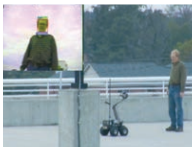
ODU's MarcBot autonomous robot performing tracking and (inset) facial recognition.
